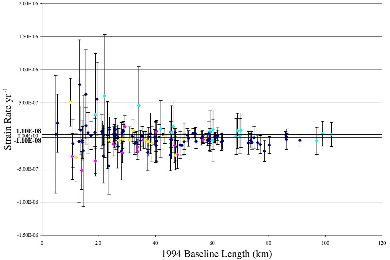
**Figure 5.** Linear baseline vectors plotted relative to their length from all stations including Awendaw 2 (AWDW) with the upper bound  $1.10\text{E-}08$  plotted. Blue diamonds are baselines that include station AWDW, the yellow diamonds are those baselines that include station RUDD and the purple diamonds are those baselines that include station CAMP.
