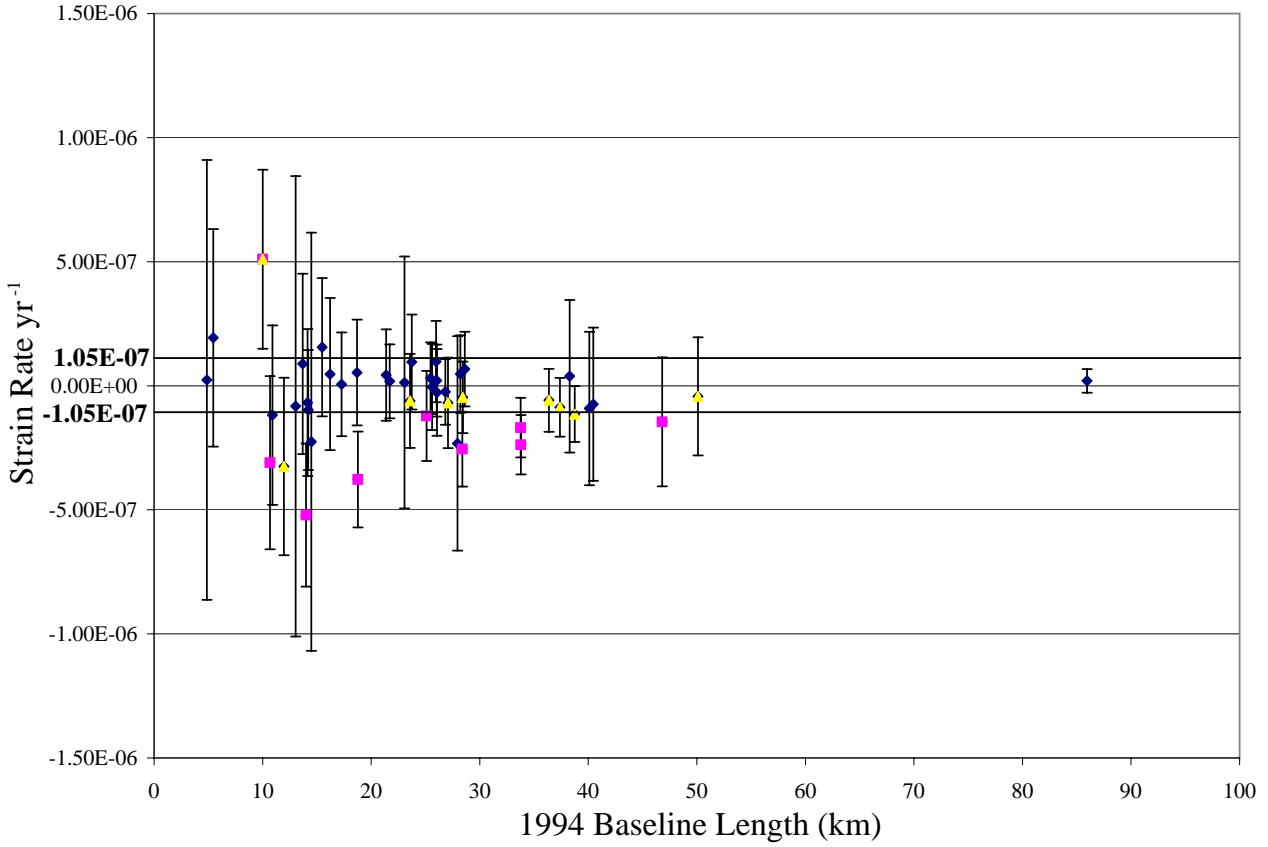
**Figure 4.** Linear baseline vectors strain plotted relative to their length from the nine stations within and around the regional sub-network with the upper bound  $1.05\text{E-}07$  plotted as thick black lines. The squares are those baselines that include station CAMP and the triangles are those baselines that include station RUDD
