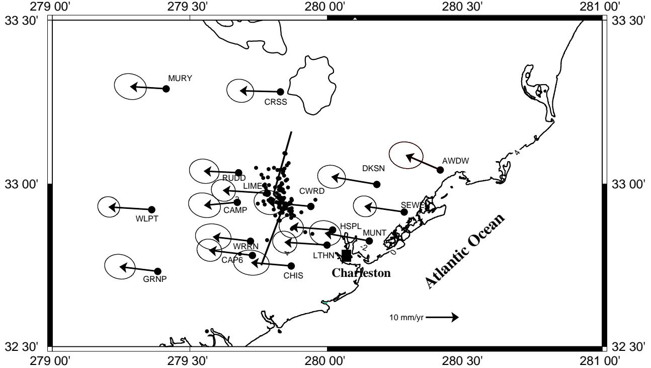
**Figure 2.** Horizontal velocity vectors with  $2\sigma$  errors in mm/yr relative to the ITRF96 reference frame. Small black dots concentrated around the fault intersection indicate the location of recent microseismicity.
