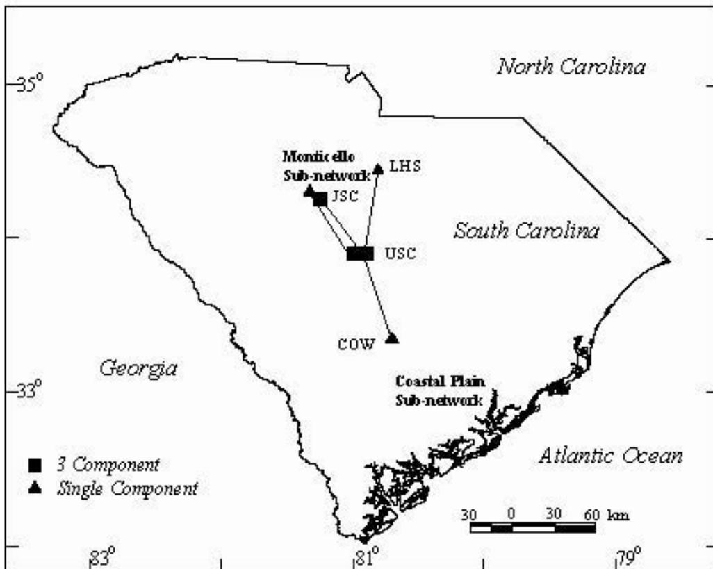
**Figure 12:** Telemetry routes for seismic data transmitted to USC.
